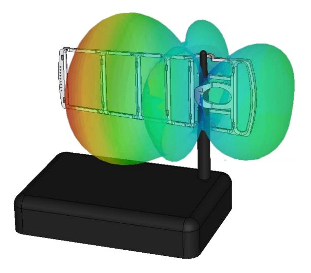
WIFI LADDER IS 7-ELEMENT YAGI ANTENNA. IT HAS DIRECTIONAL FEATURES AND AMPLIFIES TRANSMITTED WIFI SIGNAL TOWARDS SPECIFIED DIRECTION.
