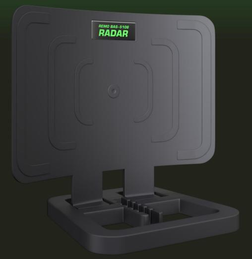
Depending on design, the antenna may be fed with coax cable directly from digital receiver, or TV-set with DVB-T2 tuner, or from USB injector that may be connected to the TV USB port or to USB port of the power supply unit.
