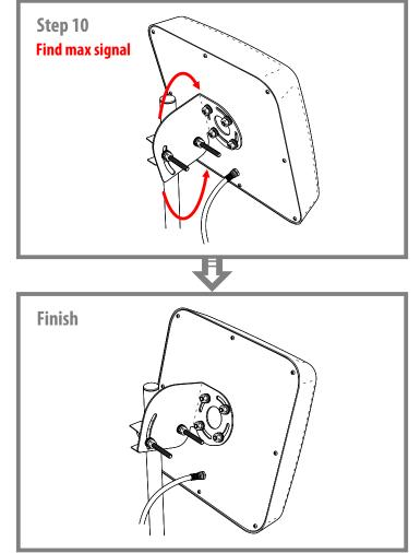
Great! You have installed the antenna and pluged it to the TV. Note - antenna does not require power.
